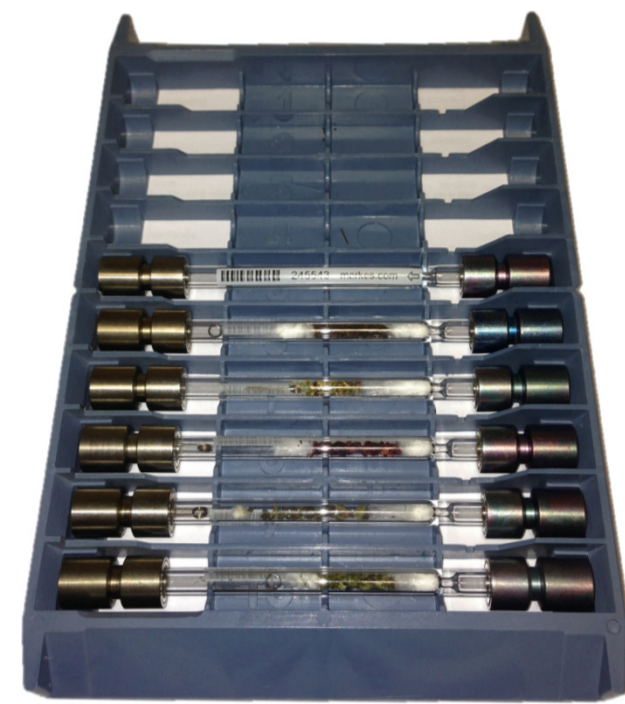
Figure 1: TD-100 tray with glass tubes containing tea leaves.
