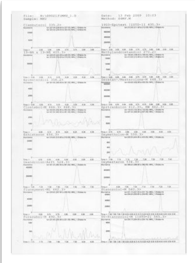
Agilent MSD ChemStation Data Analysis custom report used for analysis of banned substances or its metabolites in urine.
