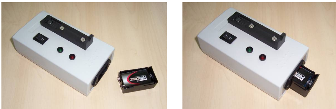
Figure 3: Inserting the 9V battery into your TAG SCRIBE
