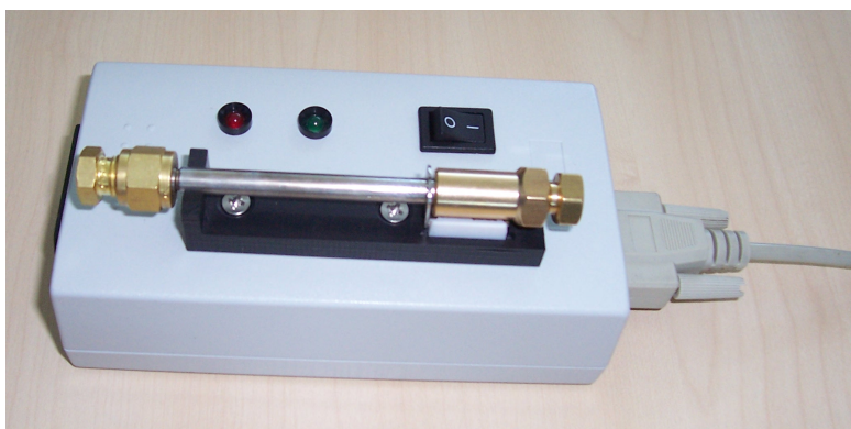
Figure 4: Tube loaded on TAG SCRIBE and TAG SCRIBE switched on
