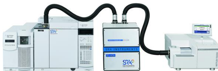
Fig. 1 – TGA-IST16-GC-MS coupling technique
