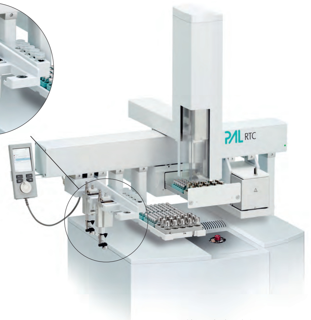
PAL RTC with standard x-axis for GC & GC/MS
