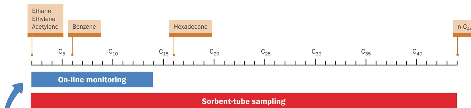
**Method-compliant analysis** is routine using the Air Server-xr. On-line monitoring can be conducted in accordance with protocols such as the US EPA PAMS scheme or the EU Clean Air Act. Sorbent-tube sampling can be performed in compliance with a number of methods including US EPA Method TO-17 or Chinese EPA Method HJ 644.
