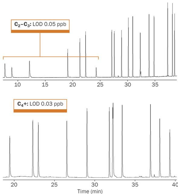
The efficient operation of the Air Server-xr provides limits of detection (LODs) well below the 0.5 ppb required, for ozone precursors ranging from acetylene to trimethylbenzene.
