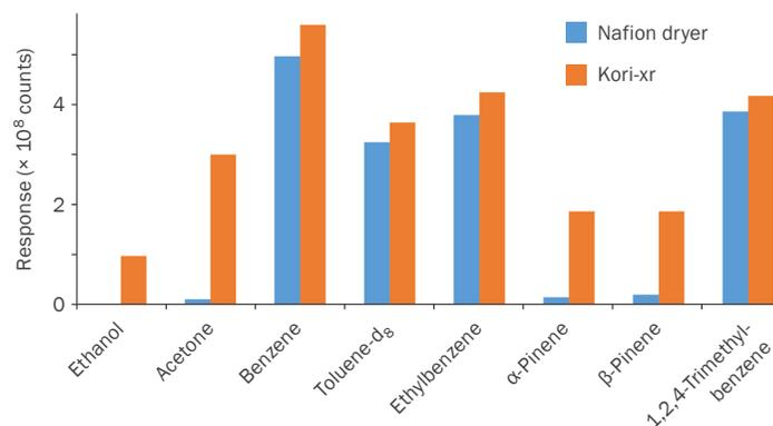
**Kori-xr shows enhanced recovery of low-boiling and polar VOCs** from an air stream with 80% RH, compared to use of a Nafion™ dryer. Kori-xr was developed in collaboration with the University of York under a Knowledge Transfer Program.
