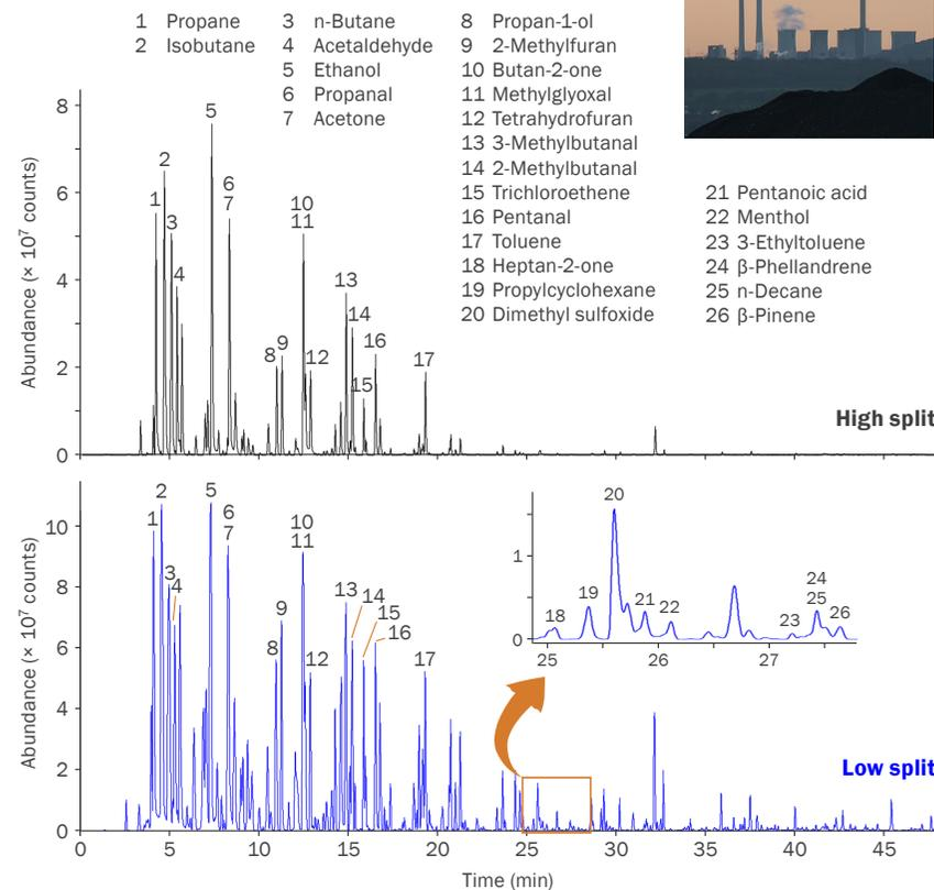
**Markes' sample splitting and re-collection technology** allows samples such as this odorous industrial air to be re-analysed. As well as aiding method validation and offering greater peace-of-mind, it also allows a single sample to be analysed at different split ratios, allowing both high- and low-concentration components to be accurately quantitated.
