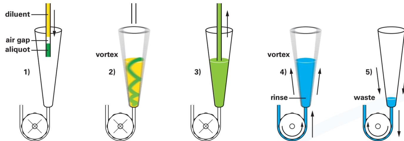
(1) aliquot and diluent are delivered to the vessel (2) vessel is mixed (3) dilution is sampled (4) fresh rinse is added and mixed (5) waste is pumped away
