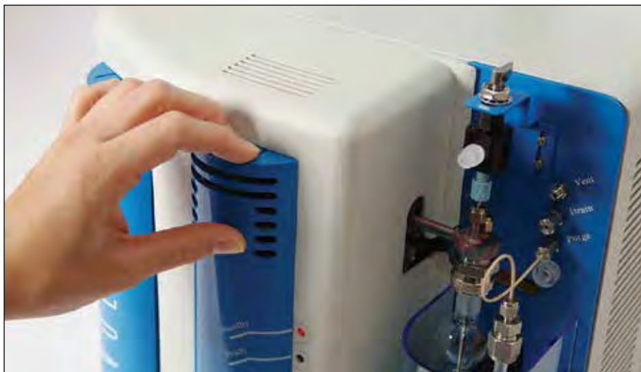
Changing traps is easy with access from the front of the instrument
