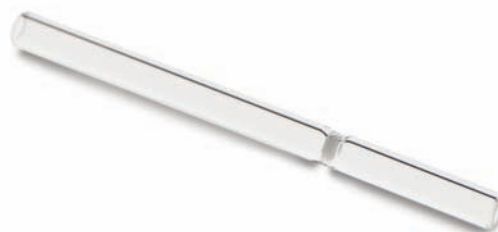
Glass tube with restriction at 30 mm – Ideal for direct desorption
