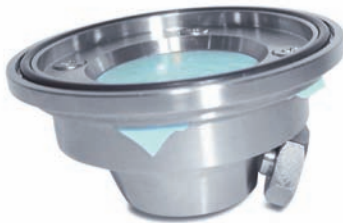
Latex sample secured in the permeation accessory
