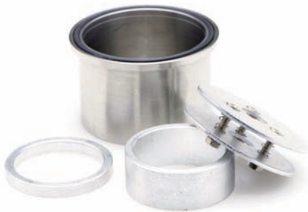
Adjustable sprung spacers for correctly positioning rigid planar materials within the Micro-Chamber/Thermal Extractor
