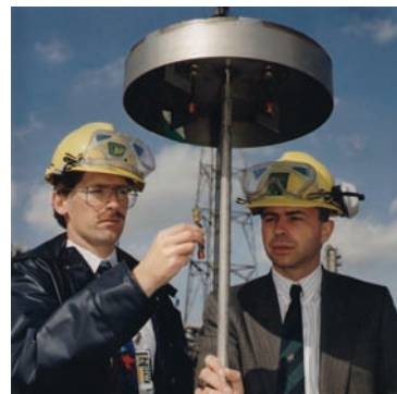
Deploying diffusive samplers for fence-line monitoring.
