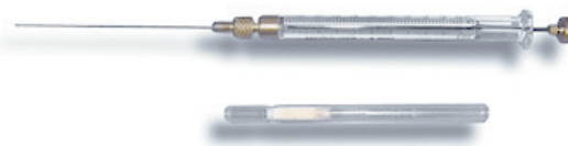
Syringe (top) and liquid-phase calibration tube containing a 1 cm bed of Tenax TA (bottom)
