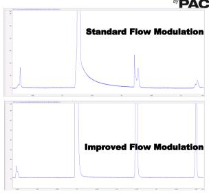
Figure 2a and 2b. Examples of Standard Flow Modulation (top chromatogram) and improved Flow Modulation (bottom chromatogram) of Cyclohexane
