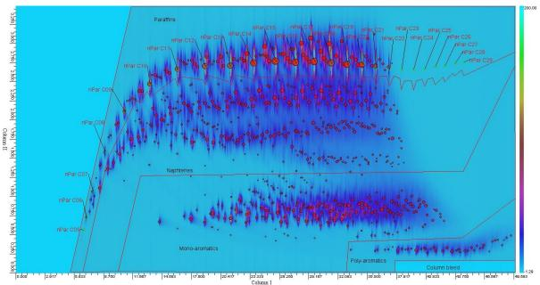
Figure 1. Typical 2D-plot of diesel sample
