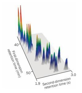
The high spectral acquisition rate of BenchTOF results in excellent peak shape and peak-to-peak resolution for challenging GC×GC analyses, such as this set of dichloroto heptachlorobiphenyls.
