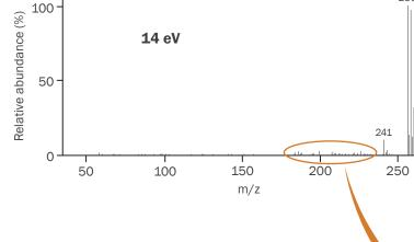
The speed and sub-amu selectivity offered by every BenchTOF is complemented by the ability of Select-eV to detect and visualise co-eluting components. In this GC×GC analysis of PCB-29, the complexity of the 70 eV spectrum makes it difficult to visualise minor impurities. The reduced fragmentation at 14 eV makes it easy to detect and deconvolve these components.
