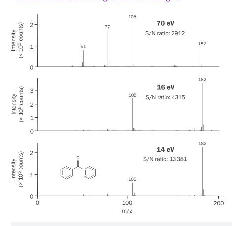
The ability of Select-eV to enhance the molecular ion stands out in this set of spectra for benzophenone (MW 182). Note the enhancement of sensitivity at lower ionisation energies, and the ability to optimise intensities of fragment or molecular ions by a slight change in the energy used for soft ionisation.
