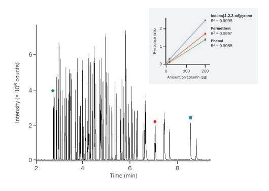
This 95-component mix of environmental contaminants and pesticides (20 pg on-column) was analysed in less than 10 minutes using BenchTOF. The inset demonstrates that excellent linearity was obtained across the analyte range. The mean signal-to-noise ratio for all 95 compounds in the 20 pg standard was 2252 and in the associated 2 pg standard was 719.
