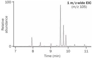
Sub-amu selectivity can eliminate matrix interferences, allowing precise identification of target compounds, as illustrated here for the emission profile of plastics used in a car stereo.
