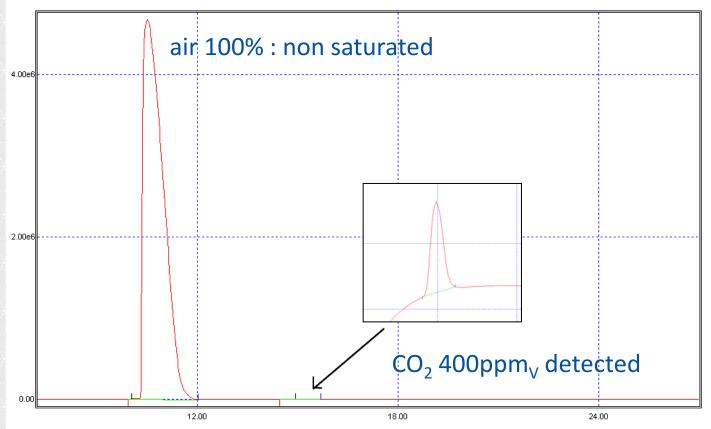
This application illustrates the large dynamic range of detector : air 100% and  $CO_2$  at very low level on the same chromatogram. It is also possible to program TCD in high sensitivity for the second peak.
