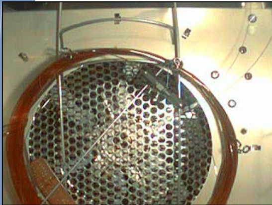
Standard installation of the column at the injection port
