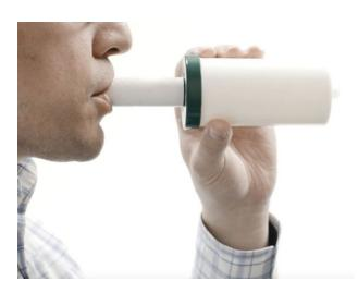
To collect a breath sample using BioVOC-2, the subject simply breathes into the disposable cardboard mouthpiece.
