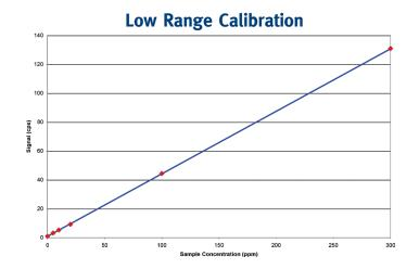
Sindie uses a weighted least squares regression in low range which is extremely linear and easy to set up. Typical correlation (R value) is expected to be on the order of 0.999 or better.
