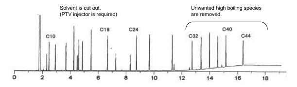
Detector contaminations are minimized by eliminating unwanted solvents such as TMS agent, etc. This is extremely useful in ECD and GC/MS experiments. Removing high boiling species results in significant reduction of analysis time and column baking time, leading to extended life of separation columns.
