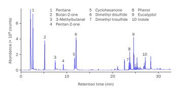
**In homeland security and forensic applications**, TD is used to detect a wide range of analytically challenging chemicals – including chemical agents, explosives, drugs of abuse, fire accelerants, and products of body decomposition (shown above).
