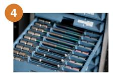
**Analysis:** The HiSorb probe is inserted into a standard TD tube for analysis by TD-GC-MS.
