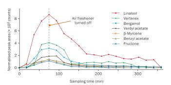
**Analysis of fragranced products** is another important application of TD, and Markes' on-line systems offer the additional advantage of continuous monitoring. This is used here to track changes in airborne components from a plug-in air-freshener.
