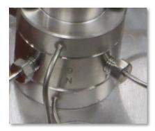
One of the challenges in the actual analysis is the possible introduction of air through valve switching. When switching a rotary valve, a very small amount of air may be directed into the columns or one of the other valve connections. This introduced air can elute from the columns together with other components. PAC has developed a valve housing in which the switching parts of the valve are covered with a helium blanket, minimizing the air introduction through the valves.
