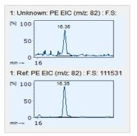
EICs (extracted ion chromatograms) of unknown sample (top) and the reference polymer in the library (bottom)
