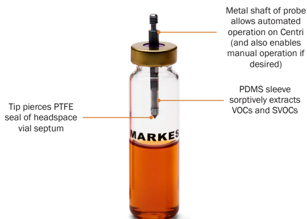
Figure 1: Short-length HiSorb probe, shown ready for headspace extraction above a liquid in a 20 mL vial. Probe desorption, followed by washing, drying and trap-based pre-concentration, are all carried out automatically on the Centri platform prior to GC-MS injection.
