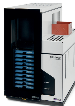
Markes' TD100-xr for automated PFAS analysis of up to 100 sorbent-tube samples.
