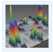
Enhanced separation by GC×GC using INSIGHT® modulation for full sample characterisation.
