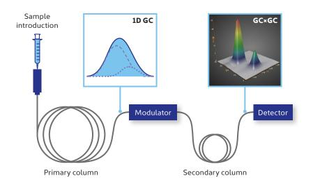
A typical analytical system for GC×GC, showing how the modulator has a central role in coupling the primary and secondary columns, and so enabling the separation of two peaks that have overlapped in 1D GC.
