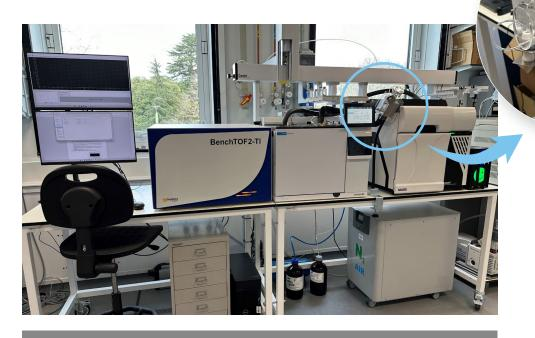
A custom-built SepSolve system at the University of Reading (UK) for advanced analytical and sensory characterisation of food. The setup comprises Markes International's Centri® extraction and enrichment platform, SepSolve's own INSIGHT-Flow GC×GC and BenchTOF2™ time-of-flight mass spectrometer, and an olfactometry port from GL Sciences.
