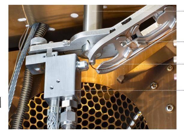
**Cryogen-free cold jet** compatible with a wide volatility range (C<sub>7</sub> to C<sub>50+</sub>).
