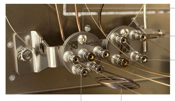
Innovative design to ensure the widest possible volatility range ( $C_1$  to  $C_{60}$ ), and the flexibility to perform heart-cutting, splitting for parallel detection or backflushing.
