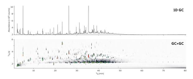
For this complex sample, GC×GC resolves about 10 times as many compounds as 1D GC – typical of the improvement in separating power that a well-chosen modulator can provide.
